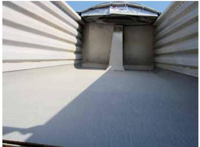
When spec'ing a tipper, choosing a versatile and durable material is essential for a smooth unloading process – not only for the actual tray, but also for the floor lining inside. E-Plas' QuickSilver floor liner is a popular option in that regard.
