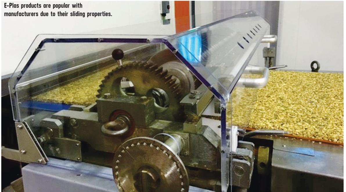
without lubrication. There is no drag and that’s because there are special additives in some of these higher spec materials that create less wear. We use TIVAR HPV material when we manufacture conveyor tracks.
