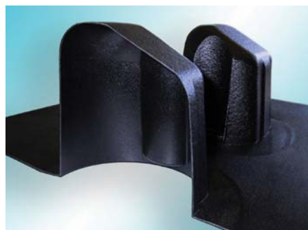
Even wall thickness of the vacuum formable nylon sheet was maintained at an extreme expansion ratio of five.
